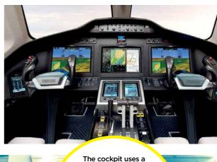
next-generation, allglass Garmin G3000 touchscreen avionics system, resulting in much more space for the pilots to fly comfortably. Also, the decrease in instrumentation means that there's more space for windows, which increases visibility.
